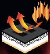
When exposed to a heat source Firecheck forms a carbonised shield deflecting heat
